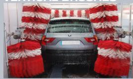
In installations from 12.5 meters, two additional vertical brushes can be installed to offer added value to the facility and higher wash quality.
