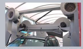
The dryer module is composed of 4 turbofans with 4 kW power each, working at low speed (1500 rpm) and with a high airflow rate for performance.
