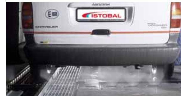
Mod. 4020600 UNDERCHASSIS WASH 10/15 BAR 160 L/M Consists of pipes with nozzles at right angles to the bay and installed below ground level. Requires water pump Mod. 4004700 or 4026400.
